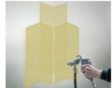
with **vertical** passes with a 50% overlap on each stroke. Leave the fluid pressure the same but lower the air pressure to match the control sample.
