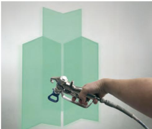
1-2 second trigger bursts per spray stroke. Use a steady motion and keep a 50% overlap on each stroke. Horizontal and vertical passes are applied wet on wet.
